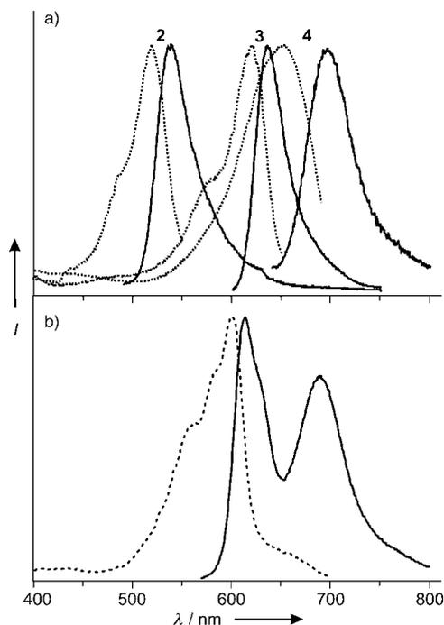
**Figure 4.** a) Excitation (dotted) and emission (solid) spectra of dyes **2** (ATTO520), **3** (ATTO610), and **4** (ATTO680) attached to zeolite L channel entrances. b) Excitation (dotted) and emission (solid) spectra of ATTO680, Ox<sup>+</sup>-zeolite L. The emission spectrum was recorded when Ox<sup>+</sup> was excited selectively at 540 nm. The excitation spectrum was recorded at 720 nm, where essentially only ATTO680 emits.
