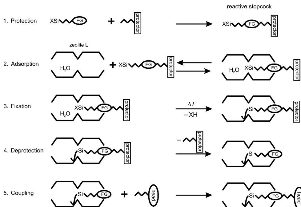
**Figure 2.** Reaction principle for the irreversible functionalization of the channel entrances of zeolite L crystals. FG: desired group to functionalize the channel ends; protector: the part of the molecule that is too big to enter the channels and that can be removed afterwards; XSi: the group that can penetrate the channels and bind to the zeolite L framework; head: the FG can be further reacted with a head if desired.
