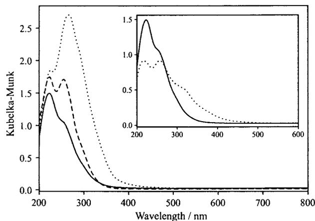
**Figure 2.** UV/vis absorption spectra of  $\text{Ag}_2\text{S}\text{--NaA-}0.05$  (solid line),  $\text{Ag}_2\text{S}\text{--NaA-}0.10$  (dashed line), and  $\text{Ag}_2\text{S}\text{--NaA-}0.50$  (dotted line) before exposure to ambient conditions. The inset shows the spectrum of freshly synthesized  $\text{Ag}_2\text{S}\text{--NaA-}0.05$  under inert atmosphere (solid line) and after 3 h under ambient conditions (dotted line).
