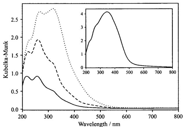
**Figure 3.** UV/vis absorption spectra of  $\text{Ag}_2\text{S}\text{--NaA-}0.05$  (solid line),  $\text{Ag}_2\text{S}\text{--NaA-}0.10$  (dashed line), and  $\text{Ag}_2\text{S}\text{--NaA-}0.50$  (dotted line) after completion of the cluster growth process described in the text. The inset shows the spectrum of  $\text{Ag}_2\text{S}\text{--NaA-}2.00$ . In this case the low energy band is already observed before exposure to ambient conditions.
