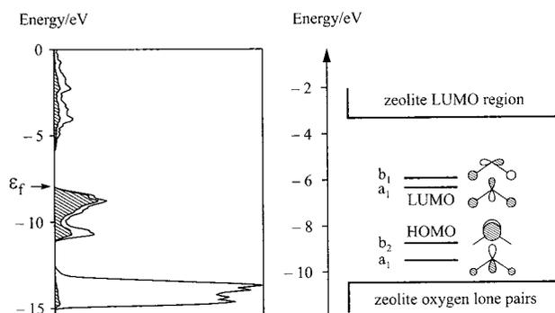
**Figure 1.** Left: Density of states (DOS) plot of  $\alpha$ -Ag<sub>2</sub>S. The hatched region indicates the contribution of sulfur 3p-states (BICON–CEDiT<sup>5</sup> calculation). The Fermi level  $\epsilon_f$  is marked by an arrow. Right: HOMO–LUMO region of a hypothetical Ag<sub>2</sub>S molecule in comparison to the HOMO–LUMO region of zeolite A (ICON–EDiT<sup>6</sup> calculation).
